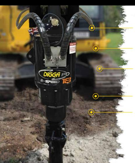
**Drill large diameter holes** with the high torque / low speed setting. Great for drilling into rock.
